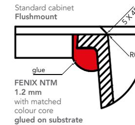
*Various machining and scoring operations can be carried out on FENIX matched colour core panels. However, please note that the scoring will alter the FENIX surface structure and lead to the loss of all specific characteristics of the product.*
